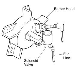
Figure 13 - Fuel Line at Solenoid Valve
